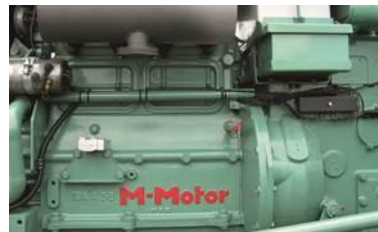
The development of the combustion chamber in the middle ball or M engine permitted softer combustion, resulting in it being nicknamed the "whispering engine".
