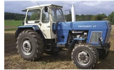
The ZT 300, the forefather of a long series of tractors in the GDR, uses MAN's M process under license.
