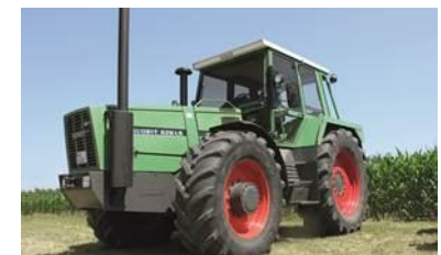
With the Favorit 622 LS and 626 LS, known as the "Coati", Fendt broke the 200 HP mark with a six-cylinder MAN engine.
