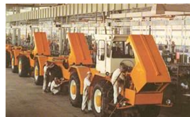
The four-wheel drive Rába 250 tow tractor sets new standards as one of the most-built articulated tractors with a MAN engine built under licence in the Eastern bloc.
