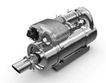
Modular EAT (exhaust gas aftertreatment) consisting of SCR mixer and SCR catalytic converter. The D4276 with 581 kW does not need DOC/DPF modules (diesel oxidation catalytic converter/diesel particulate filter) to comply with EU Stage V and US Tier 4.
