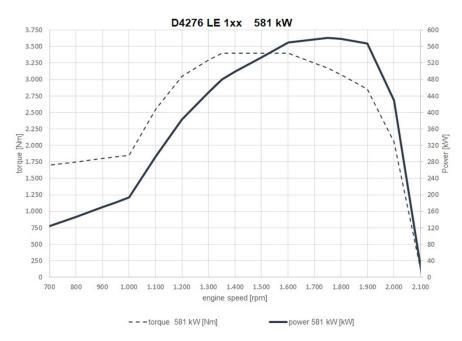
A newly developed charging concept ensures that the D4276 has a large power output and torque values in the high engine speed ranges.
