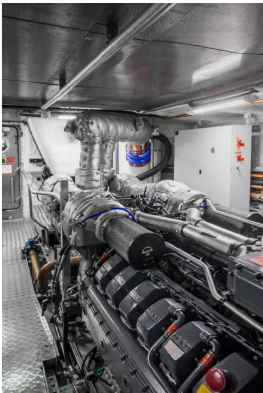
*Two MAN D2862 LE469 field trial engines rated for 1,029 kW (1,400 hp) at 2,100 rpm, including a modular exhaust gas aftertreatment system. These were successfully used in the pilot boat Luna at the Port of Rotterdam.*
